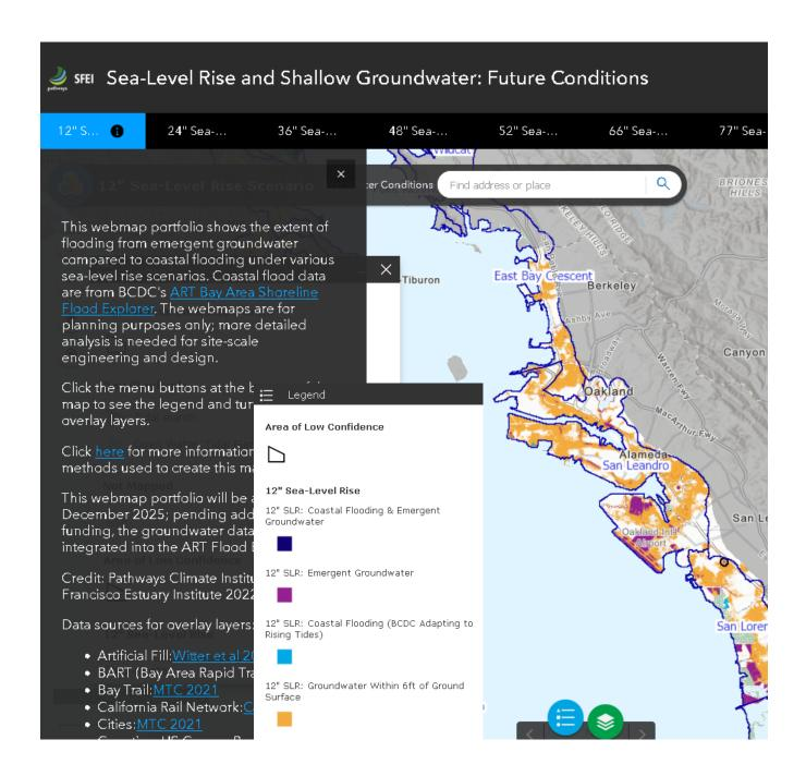
Preliminary predictions of groundwater conditions with 12" of sea level rise. Gray = not mapped, white = low confidence, orange = groundwater within 6 ft. of ground surface...
